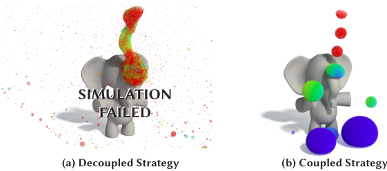
Fig. 11. Surface-tension-dominated fluids (velocities are color-coded). (a) Decoupled treatment of surface tension, viscosity, and incompressibility leads to numerical instability. (b) Our unified method with strong coupling of all three effects ensures stable and robust simulation.
